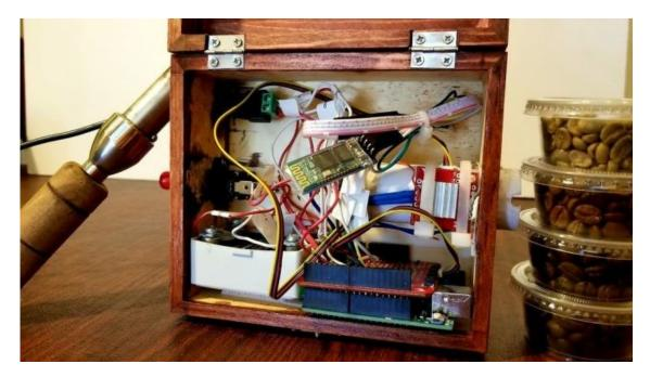
While you may not consider in detail how your coffee is roasted, those that produce it must pay special attention to make sure that the end product is consistent. Equipment to help analyze roasted coffee is normally quite expensive, but using a near-infrared sensor, <u>Arduino Uno</u> and Bluetooth module, Spencer Corry was able to make his own <u>analysis setup</u>.
